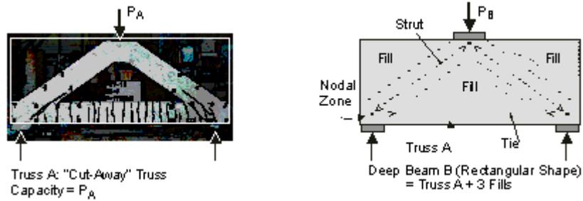
**Figure 4** Illustration of “Cut-Away” and “Filled-In” Truss
