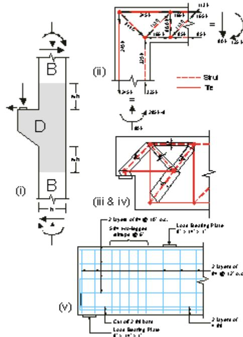
**Figure 3** Strut-and-Tie Models and Steps in Design
