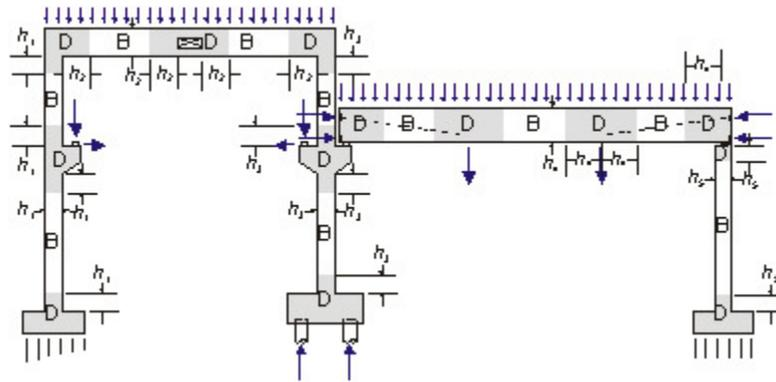
**Figure 1** Example of D-Regions in a Common Building Structure
