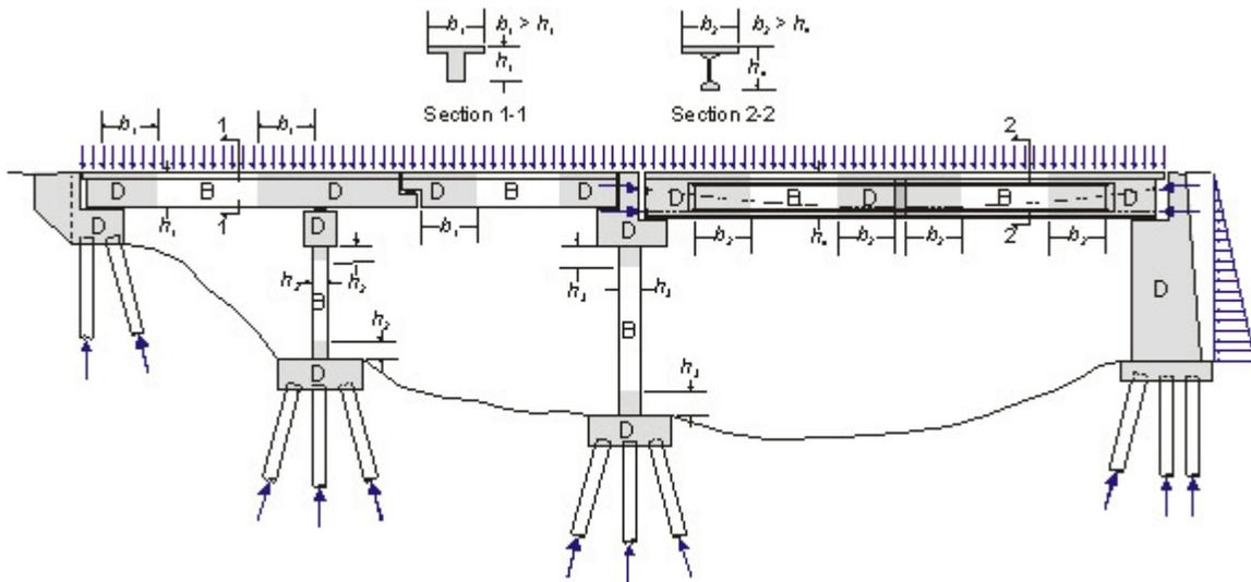
**Figure 2** Example of D-Regions in a Common Bridge Structure
