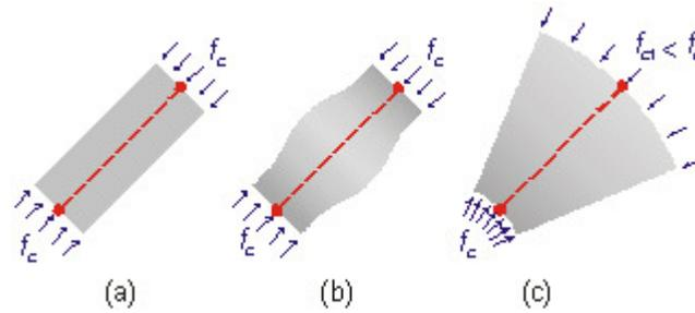
**Figure 4** Basic Type of Struts in a 2-D Member: (a) Prismatic (b) Bottle-Shaped (c) Fan-Shaped
