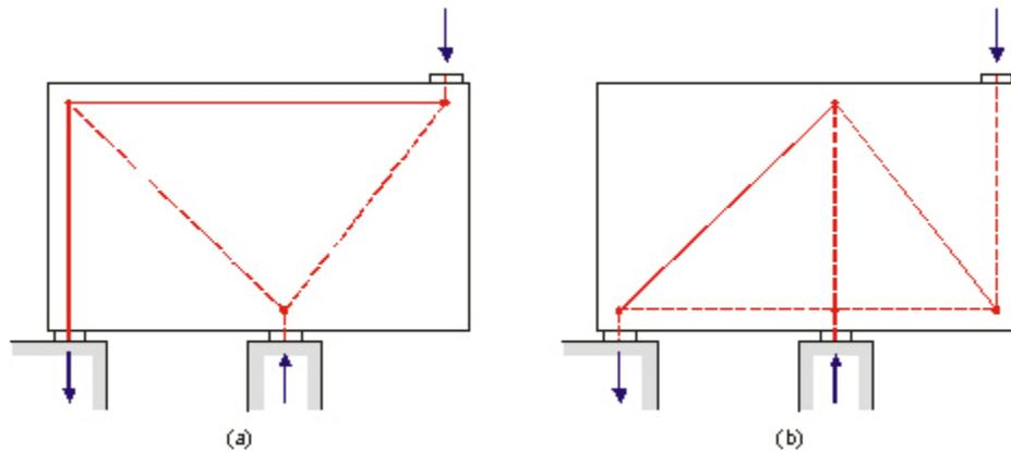
**Figure 6** Two statically admissible strut-and-tie models for a cantilevered deep beam under vertical loading: (a) Workable truss (b) Less favorable truss due to excessive ductility demands
